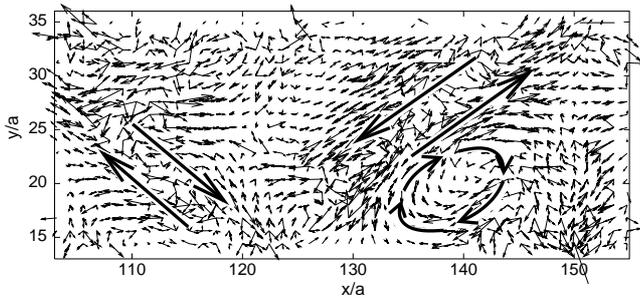
FIG. 7: In situ displacement field of the Laves crystal at  $u_p/c_l = 0.45$ . The large antiparallel arrows indicate slip planes. The ring of large arrows marks a rotation axis. Pictures of the quasicrystals look similar. The numbers at the figure represent the size in nearest neighbor distances  $a$ .
