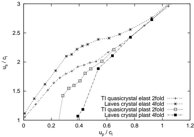
FIG. 5: Shock vs. piston velocity. At low piston velocity (quasi-)elastic behavior is observed. Between  $u_p/c_l = 0.3$  and  $0.6$  approximately a crossover to the plastic shock wave and finally the change of slope to a materials-independent value is found. The velocities  $u_p$  and  $u_s$  are scaled by the velocity of sound  $c_l$  valid for the different directions.
