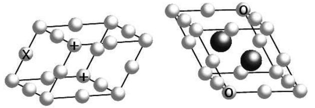
FIG. 1: Oblate and prolate rhombohedron. Light gray: small atoms, dark gray: large atoms. Left: the x marks the atom around which 10 oblate rhombohedra fit together. The atoms marked with the + form a puckered decagon, around which the ring processes occur. Right: the atoms marked with o denote the intersection points of the  $\langle 100 \rangle$  direction.
