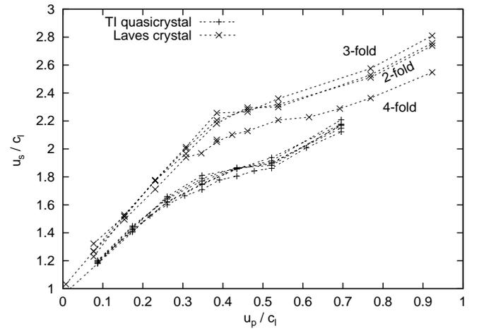
FIG. 6: Orientation dependence of the shock vs. piston velocities. The quasicrystal curves are identical if errors are taken into account. Therefore they are not marked individually. For the Laves crystal, the velocities along the 4-fold direction differ from the other orientations which on their part are again quite similar. The velocities  $u_p$  and  $u_s$  are scaled by the velocity of sound  $c_l$  valid for the different directions.
