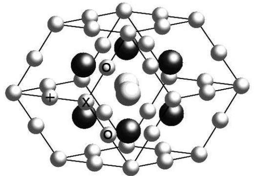
FIG. 2: The rhombic dodecahedron. The atom marked with an x and its symmetry-equivalent copies are the primary sites of flips. The large light gray atoms are also very mobile. The atoms marked with + and o are secondary sites for diffusion.
