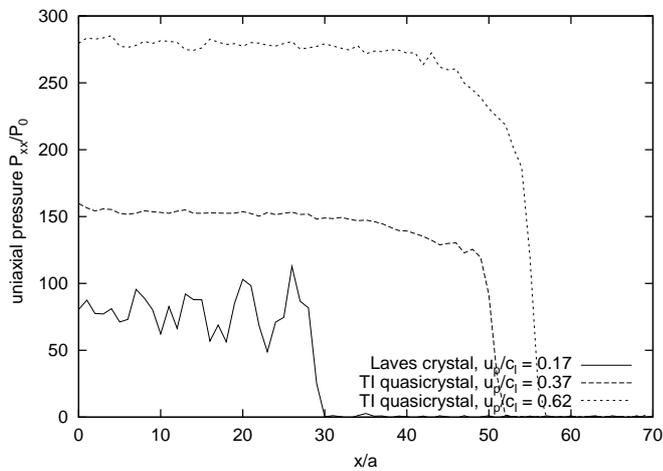
FIG. 4: Uniaxial pressure  $P_{xx}$  of three samples typical for the three regimes.
