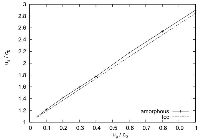
FIG. 12: Shock vs. piston velocity for the amorphous solid (dotted curve). The fcc curve (full line) is from Holian and Lomdahl<sup>13</sup>.
