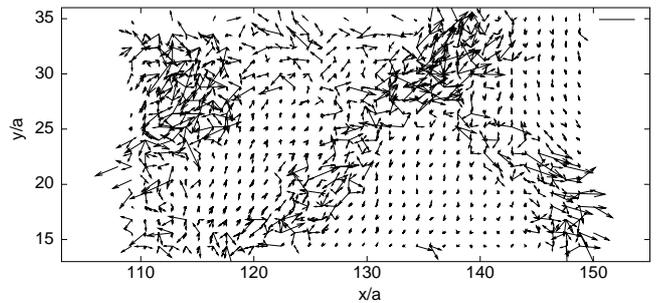
FIG. 8: Displacement field of the Laves crystal at  $u_p/c_l = 0.45$  after quenching. Shown is nearly the same part of the sample as in Fig. 7. Pictures of the quasicrystals look similar. The numbers at the figure represent the size in nearest neighbor distances  $a$ .
